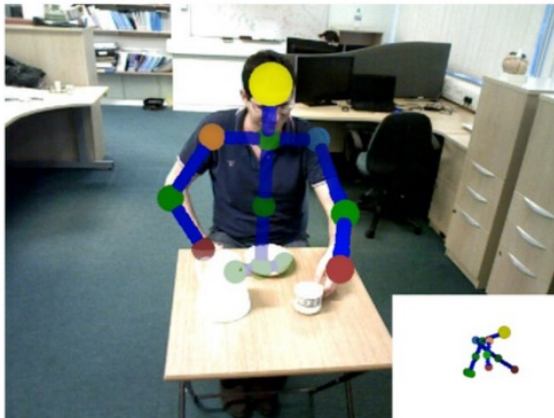
Figure 1: Activity recognition in a table top setting. Dyadic QSR relations between detected objects/skeleton points can be computed (bottom right inset).
